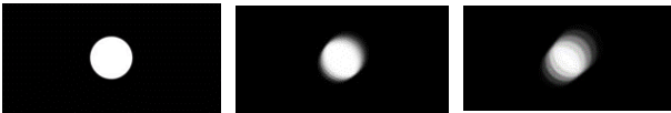
Figure 2. Blurring effect: example of radial blurring applied to a white circular dots. Left: original image without blurring. Center: blurring \rho = 0.01 Right: blurring with \rho = 0.02 .
