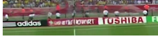
Fig. 7. The result of image in-painting. The blocked banner contents of "Frankfurt" and "Toshiba" are re-constructed.
