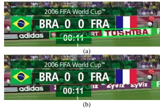
Fig. 8. The AD replacement result after image in-painting. (a) The correct banner detection. (b) The AD replacement result.
